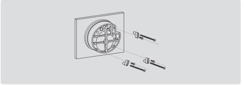
5-4) In case of surface mounting, prepare 3 holes corresponding to Instrument 3 holes which are 120° apart from each other on a circle of 103 mm.
